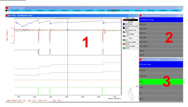
• 2 & 3 are Bit indicators. So when they switch to Green it means the corresponding outing/action is ON.
