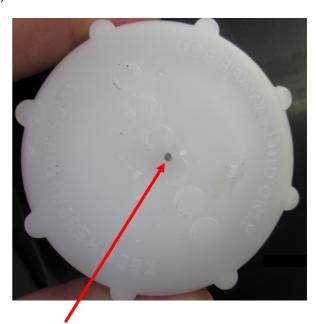
2) Drill a Ø2mm hole in the center of the cap Make sure that no plastic chip stays in the cap before re fitting
