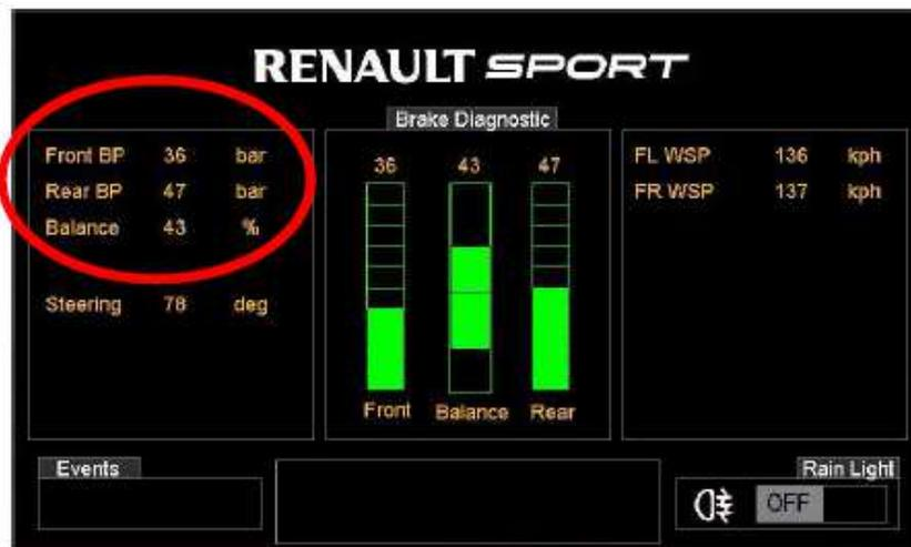
2) Tighten the rear brake pressure limiter clockwise (+) to allow the maximum pressure (must be around 40 bars)
