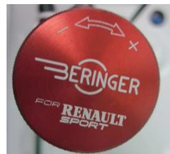
3) Adjust the position of the balance bar threaded rod by turning it (manually or using the knurling wheel) to the desired position taking into account that the brake balance (% of total pressure on front axle) must be constant till the maximum rear brake pressure is reached.
