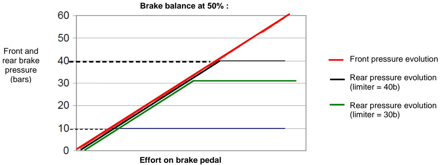
The graphics shows what you can observe in Toolbox with front and rear brake pressure sensors. As the brake balance is set at 50%, front and rear axle increase evenly when the driver touches the pedal. The rear brake pressure is limited at the defined threshold. When this threshold is reached, the pressure on the front axle keeps on increasing and the rear pressure stay stable (which modifies the brake balance).
