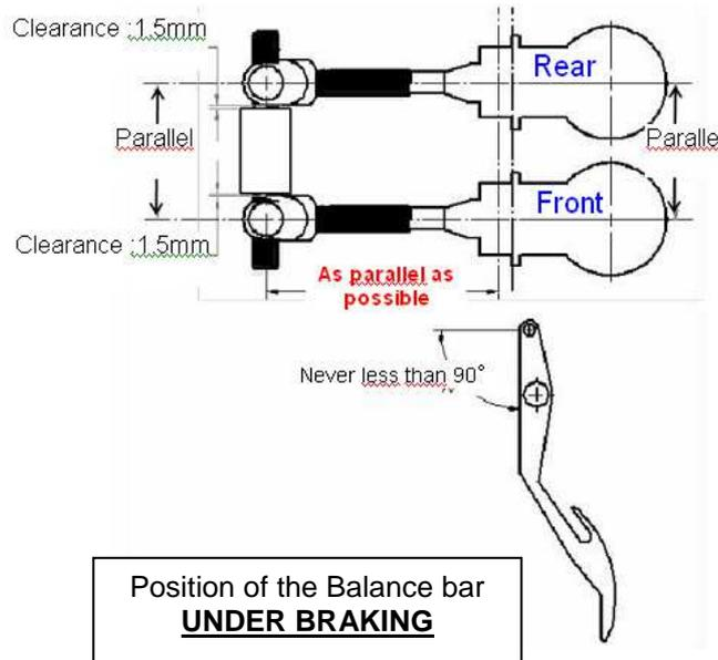
As both master cylinders have a different stroke, you have to adjust the master cylinder rod lengths with the 2 balance bar brackets at rest (the front master cylinder push rod will be longer than the rear master cylinder one of a few mm as the front master cylinder will travel more under braking). The setting should be as explained below :
