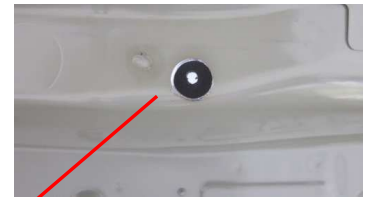
Figure 6bis : View from under the car : 2 holes Ø16mm concentric with the 2 Ø5mm
