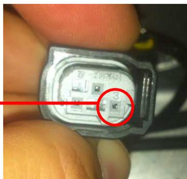
Find the wire connected to the contact n°3.
